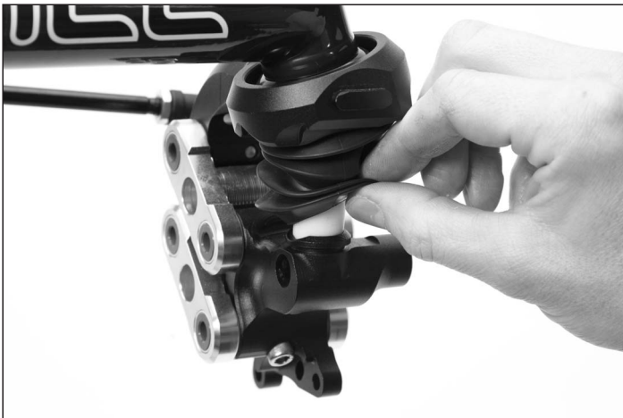
Slide off rubber gaiter at the bottom.
