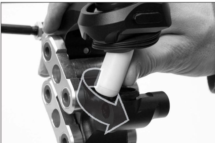
Slide bottom of elastomer around to the front of the king post.
